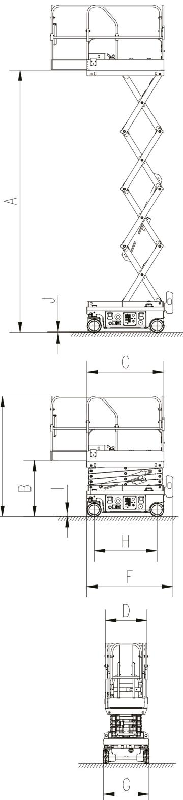
\* The working height equals to the platform height plus 2 m.
